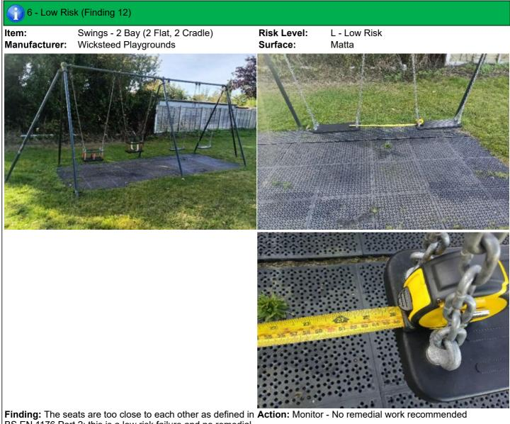
**Finding:** The seats are too close to each other as defined in **Action:** Monitor - No remedial work recommended BS EN 1176 Part 2; this is a low risk failure and no remedial action is required
