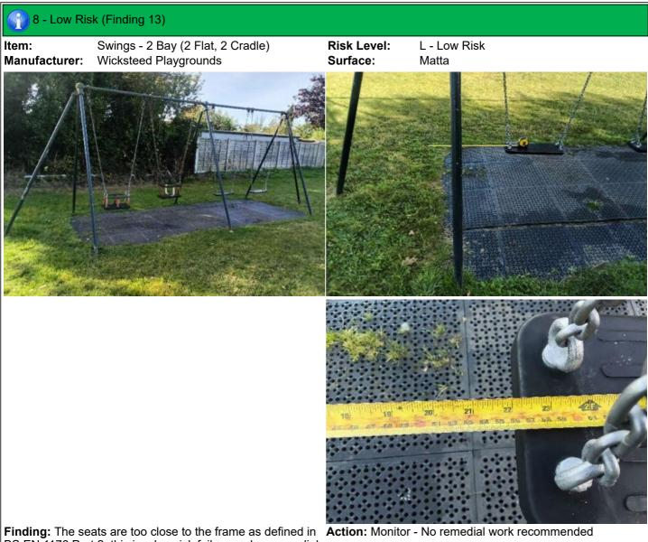
**Finding:** The seats are too close to the frame as defined in BS EN 1176 Part 2; this is a low risk failure and no remedial action is required
